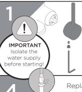
Remove cap and grub screw. Remove handle
