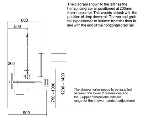
Shower controls shown must fall within the 750mm to 1000mm above the floor requirement. Positioning the centre of the Shower Diverter at the 1000mm height sets the thermostatic mixer valve at a height such that it does not interfere with the rails. Adjustability of the shower handset is greater than the required heights but should be operable between the 1200mm and 1400mm heights shown.
