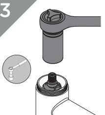
Remove the valve using the tool required for your tap.
