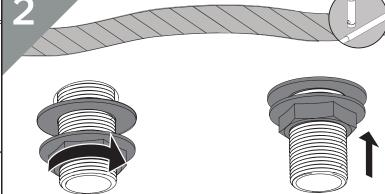
To secure the taps to the bath, use a box spanner to tighten the metal backnuts underneath ensuring the washer is correctly positioned in between the backnuts and the bath
