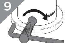
EasyFit tool and tighten the grub screws with an extra 1/2 turn.
