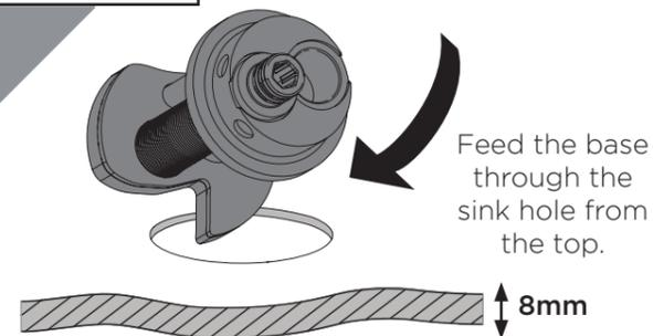
If the surface the tap is being fitted to is over 8mm; or you feel the tap needs extra stability, follow the **alternative installation steps** overleaf.
