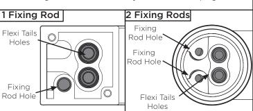
If required, thread the flexible tails and fixing kit rods through the plinth and rubber seal (if loose) and align with tap body.
