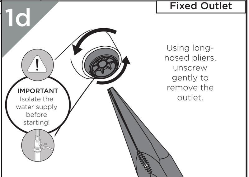
This diagram shows a tap with a fixed outlet. Long-nosed pliers are used to unscrew the outlet. A warning icon and text state that the water supply must be isolated before starting. An inset shows the pliers being used on the outlet.
