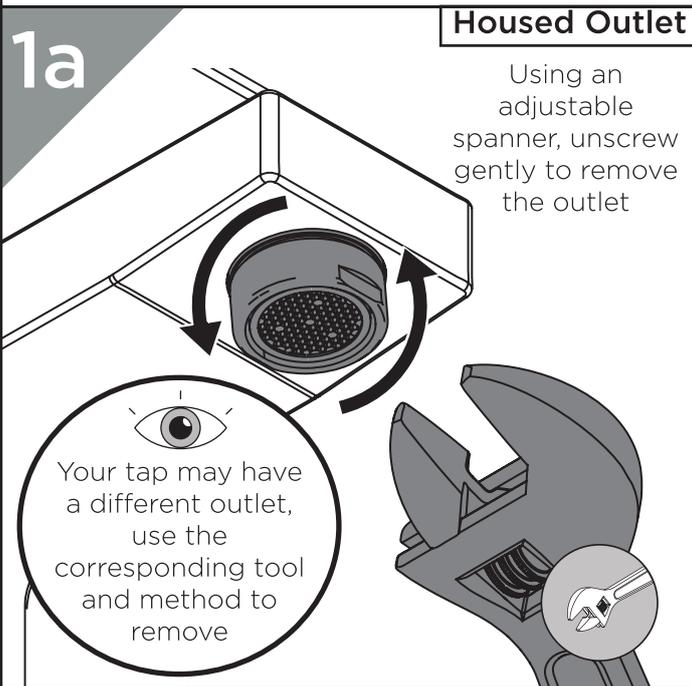
This diagram shows a tap with a housed outlet. An adjustable spanner is used to unscrew the outlet. A callout shows an eye icon and text stating that different tools may be needed for different tap models. An inset shows the spanner being used on the outlet.
