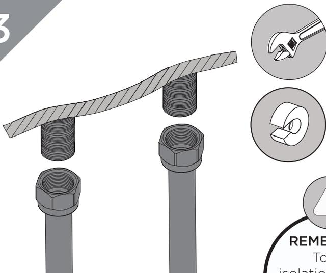
Connect the hot and cold water supplies to the threaded tails.
