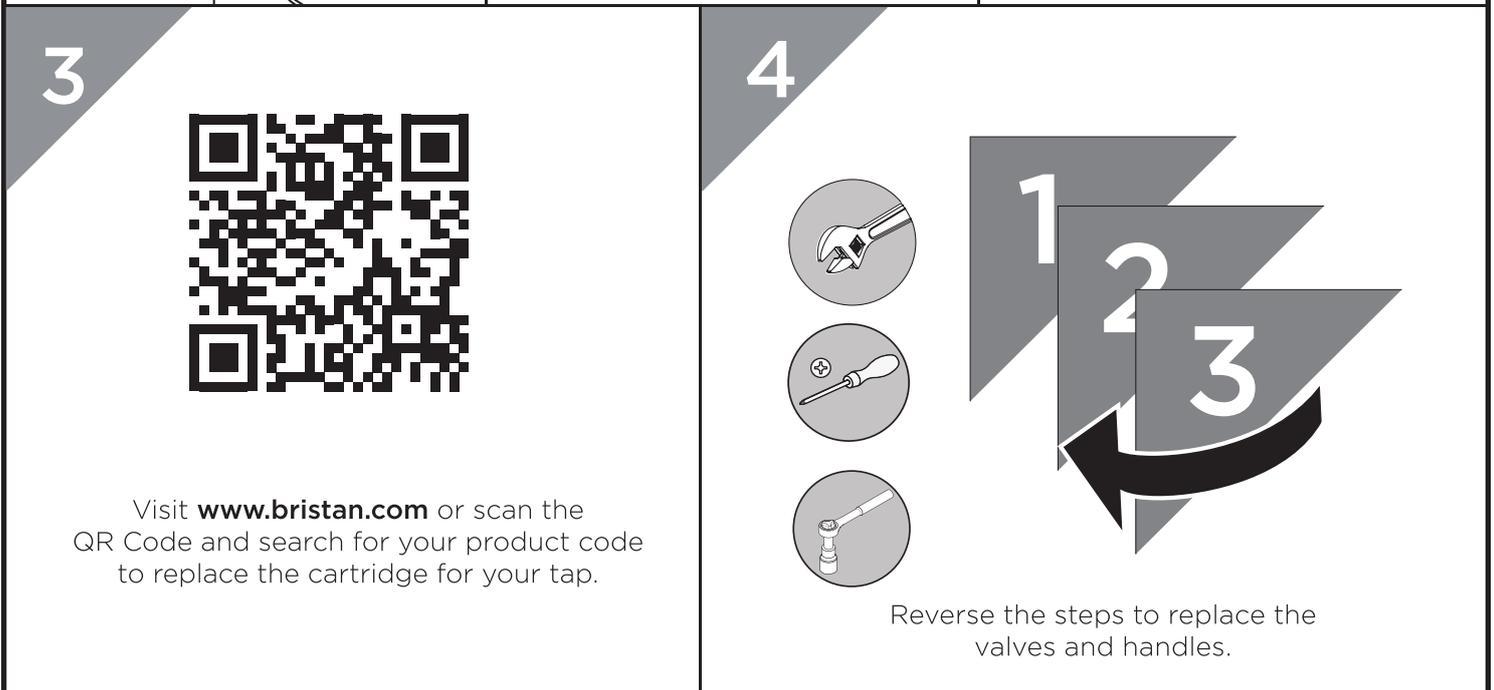
Reverse the steps to replace the valves and handles.
