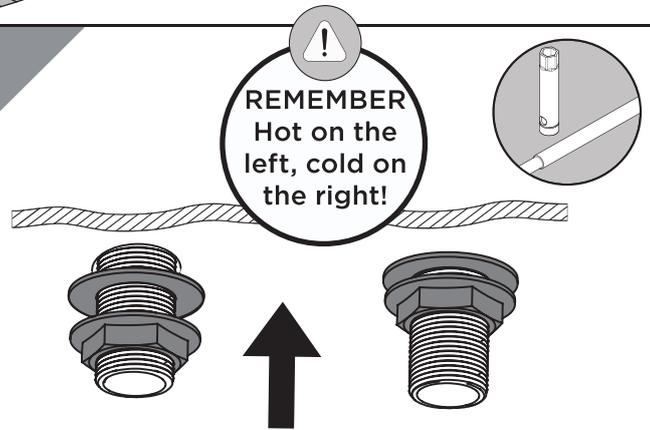
Secure the taps to the basin/bath by using the washer and metal backnut below the basin/bath.
