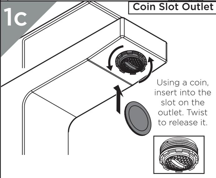
This diagram shows a tap with a coin slot outlet. A coin is inserted into the slot and twisted to release the outlet. An inset shows the coin and the removed outlet.
