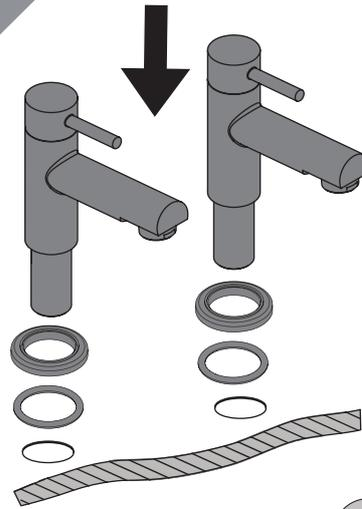
Feed the tap body through the bath/basin and ensure plinth and plinth seals are in place.
