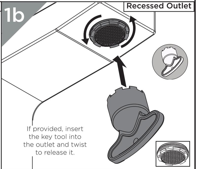
This diagram shows a tap with a recessed outlet. A key tool is inserted into the outlet and twisted to release it. An inset shows the key tool and the removed outlet.
