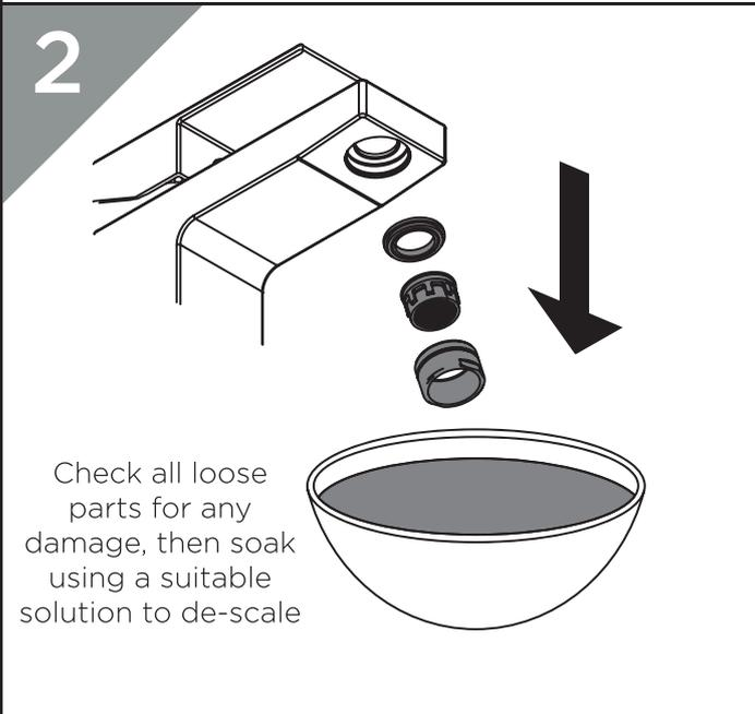
This diagram shows the disassembled parts of the tap being soaked in a bowl of solution. An arrow points from the disassembled parts to the bowl.
