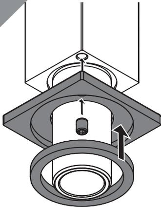
You may be required to secure the plinth to the tap with a grub screw.
