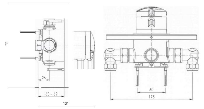
Suitable for wall cavity depths of between 60 - 69mm.
