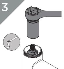
Remove the valve using the tool required for your tap.
