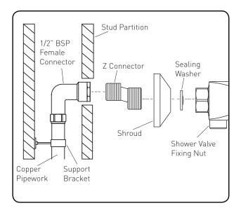
Important: When fitted the Z connectors must protrude from the shroud by 7mm + 1mm with 150 centres.
