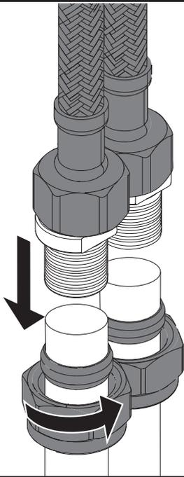
Connect the hot and cold water supplies to the flexible tails and turn until tight
