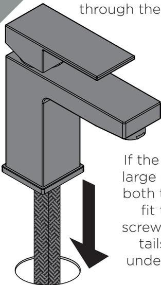
If the hole is not large enough for both tail ends to fit through, screw one of the tails in from underneath the bath
