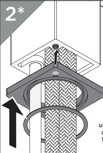
If required, thread the flexible tails and fixing kit rods through the plinth and rubber seal (if loose) and align with tap body
