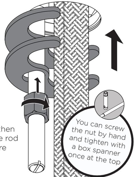
You can screw the nut by hand and tighten with a box spanner once at the top
