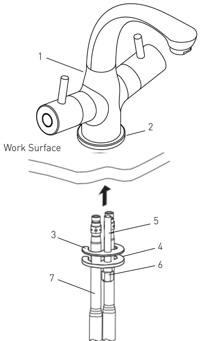
3. Screw the copper connecting pipes (7) into the mixer tap.
