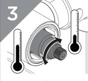
Turn the spindle anti-clockwise to increase the temperature; clockwise to decrease the temperature. Check the emperature and adjust until you achieve the desired result.
