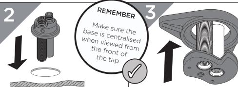
Feed the base through the sink hole from the top.
