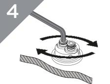
Turn the hexagonal key clockwise to secure the EasyFit Base.
