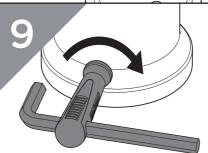
Thread the hexagonal key through the EasyFit tool and tighten the grub screws with an extra 1/2 turn.
