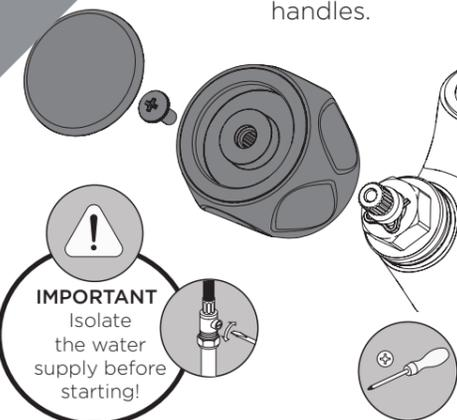
2 Remove the valves using a suitable spanner.
