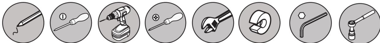
Pencil Flat head Screwdriver Drill Cross head Screwdriver Spanner Pipe Cutter Hexagonal Keys Socket Spanner
