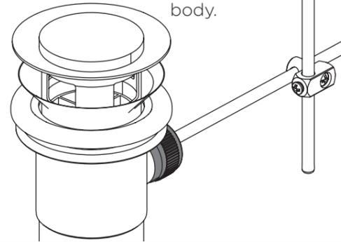
To set the plug height adjust the waste rod, operating rod, connecting bracket and the screw.
