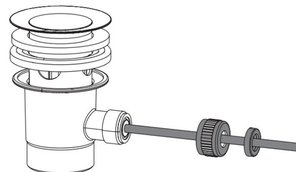
Place the washer and waste body plate onto the horizontal arm. Screw the waste body plate onto the lower waste body.
