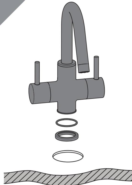
Fit the tap to the sink, including the rubber washer.
