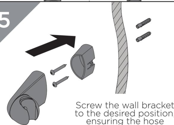
Screw the wall bracket to the desired position, ensuring the hose and handset can reach.
