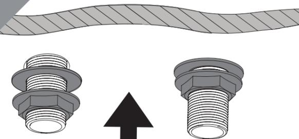
Secure the taps to the bath by using the washer and metal backnut below the bath.
