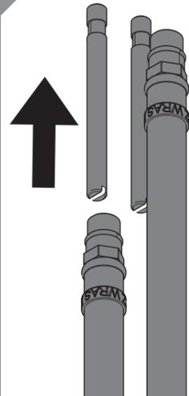
Screw in the flexible tails by hand. **DO NOT OVERTIGHTEN.**
