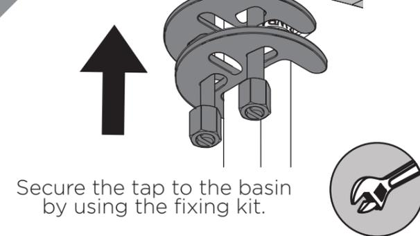
Secure the tap to the basin by using the fixing kit.
