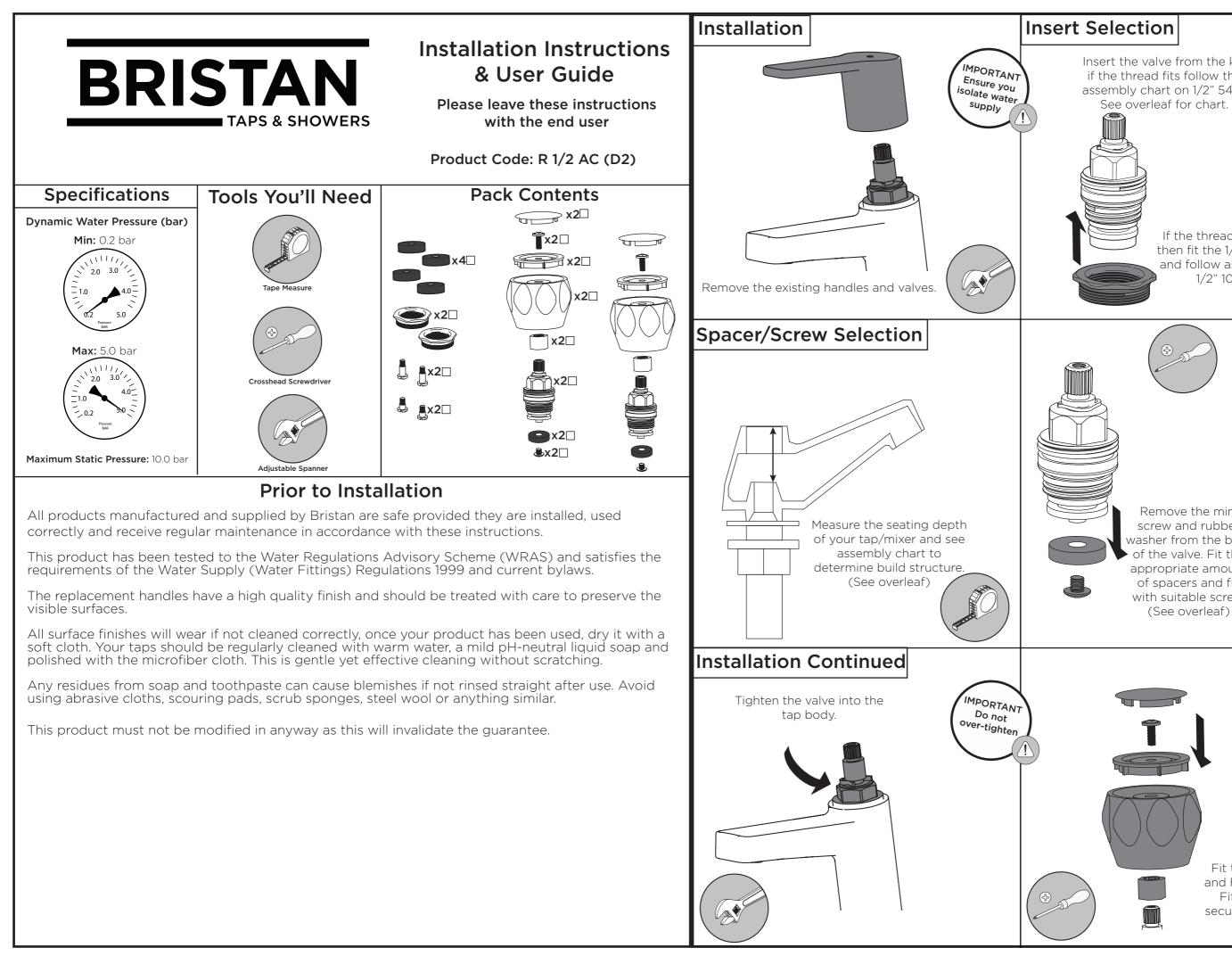
Insert the valve from the kit, if the thread fits follow the assembly chart on 1/2" 5412. See overleaf for chart.
