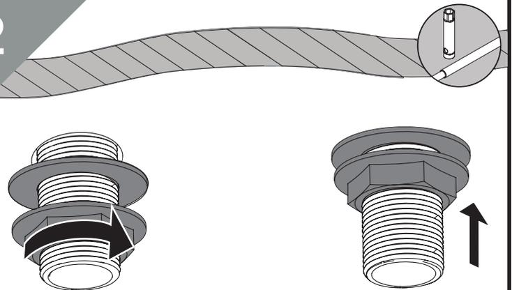
To secure the taps to the bath, use a box spanner to tighten the metal backnuts underneath ensuring the washer is correctly positioned in between the backnuts and the bath
