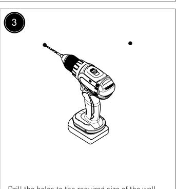
Drill the holes to the required size of the wall plugs. Insert the wall plugs into the holes. This is based on the supplied fixings being suitable for the wall. If not, obtain suitable fixings.
