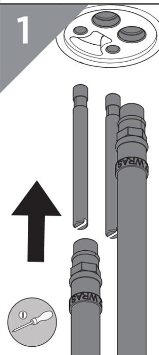
Screw in the fixing kit rods to the tap base. Screw in the flexible tails by hand only. **DO NOT OVERTIGHTEN.**
