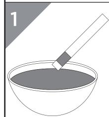
Draw a small amount of cold water. Using the test strip provided, dip into the water for 3 seconds and wait for 20 seconds to develop.
