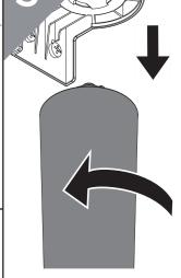
Place a small bowl underneath the filter sump and remove it.
