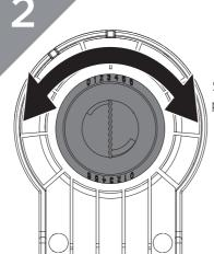
Using the result of the water test carried out in Step 1, push and turn the pre-fitted blue key to the required filter setting.
