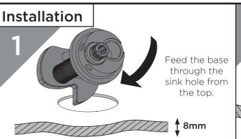
If the surface the tap is being fitted to is over 8mm; or you feel the tap needs extra stability, follow the alternative installation steps overleaf.
