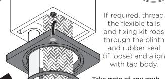
Take note of any grub screw holes on the underside of the tap and align them correctly to the holes on the plinth.
