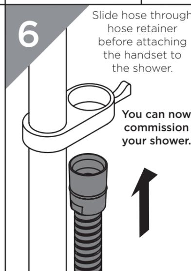
Slide hose through hose retainer before attaching the handset to the shower.
